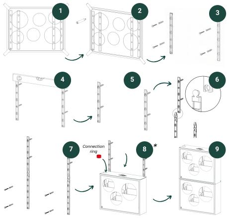
\*Always insert the connection ring into the pouring opening of the lower box.
